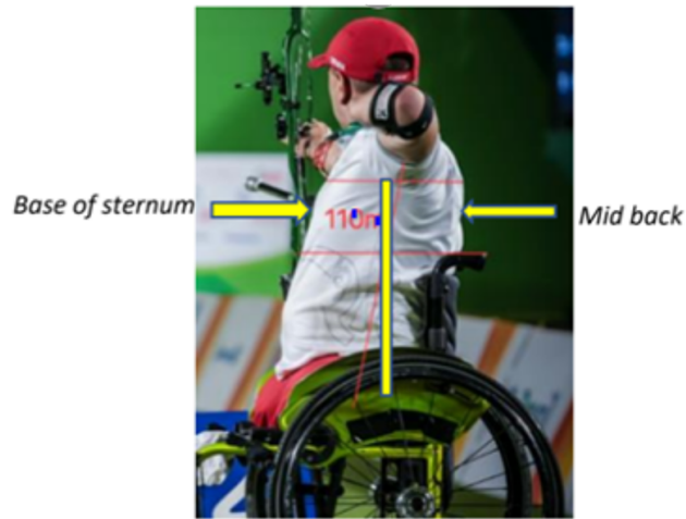
Image 19: Wheelchair lateral support measurement
